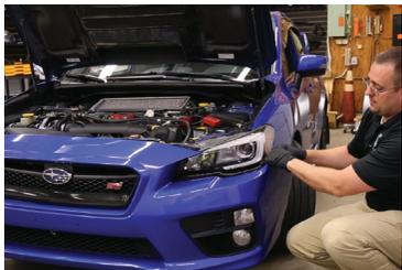
3. With the bolts and rivets removed, detach the bumper from the car by pressing the clips located along the side of the bumper below the headlight. Repeat on the other side. Pull straight back and set the bumper aside on a soft surface.
