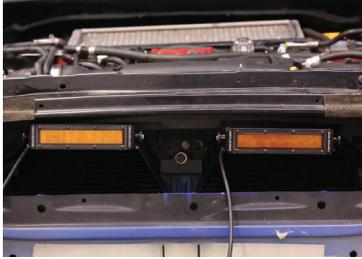
6. Using the factory mounting points, mount the bracket and replace the original screws, only hand-tightening them.
