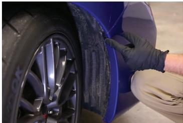
2. Next, remove the plastic rivet located between the fender and the bumper. Repeat on the other side. Then, remove the 6 plastic rivets located below the bumper.
