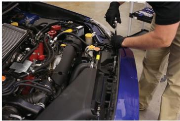
1. Using a 10mm socket and plastic trim removal tool, remove the 6 bolts and 4 plastic rivets located on the edge of the bumper inside the engine bay.
