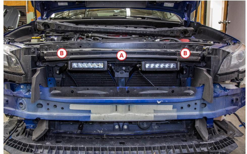
4. With the bumper removed, locate and remove the 12mm bolt **A** in the center and the two 10 mm bolts on the sides. **B**
