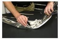
2. Bring the bezel to a soft, non-marring working surface. Then unclip the reflector lens from the bezel by squeezing the clear clips with a pair of pliers and pushing downward on them.
