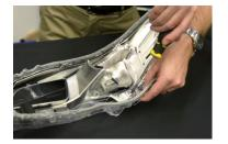
1. Remove the lens and set the headlamp assembly aside. Next, remove the 3 screws holding the bezel to the lens. Then remove the bezel from the headlight lens.
