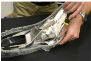
1. Remove the lens and set the headlamp assembly aside. Next, remove the 3 screws holding the bezel to the lens. Then remove the bezel from the headlight lens.
