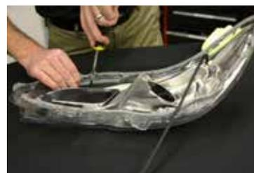
6. Using a microfiber cloth, remove any finger prints that may be on the bezel then reinstall it back into the headlight lens by clipping it into place. Reinstall the original screws.
