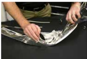
2. Bring the bezel to a soft, non-marring working surface. Then unclip the reflector lens from the bezel by squeezing the clear clips with a pair of pliers and pushing downward on them.
