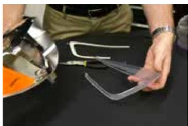
3. Pull the reflector lens straight out to remove it and set it aside.
