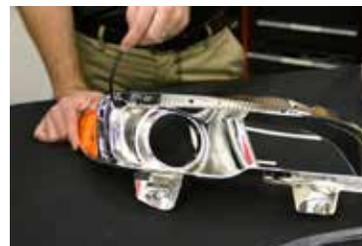
4. Install your new Diode Dynamics C-Light by running the wires through the hole where the factory bulb was and setting the LED board into place.
