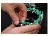
5. Pull straight up on the factory board to remove it from the shroud.
