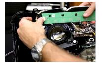
1. Remove the headlamp lens. Using a T20 Torx Screw Driver, remove the screws holding both reflector housings in place to access the factory LED panels. Pull the reflector housings away from the headlamp and unclip each connector.
