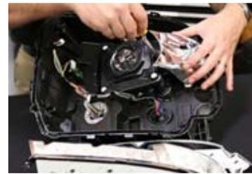
5. Next, remove the turn signal housing from the headlamp.
