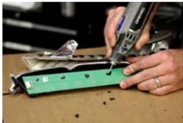
2. Take both reflector housings to a clean area. Using a rotary (Dremel) tool, remove the factory LED boards by shaving down the black plastic rivets holding the LED panels to the housing. Pull the factory board away from the housing. Repeat for all three factory boards.
