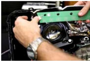
1. Remove the headlamp lens. Using a T20 Torx Screw Driver, remove the screws holding both reflector housings in place to access the factory LED panels. Pull the reflector housings away from the headlamp and unclip each connector.
