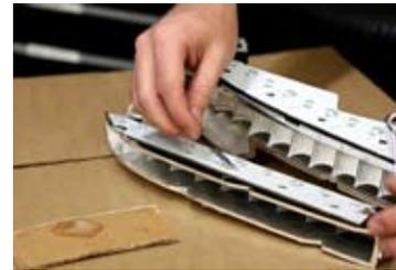
4. Fix the new panels in place by applying 5-minute epoxy to completely cover the plastic rivets tabs. The epoxy should create a bond between the plastic rivet point and the board. Use enough epoxy so that there is a bond all the way around each rivet, contacting the board fully.
