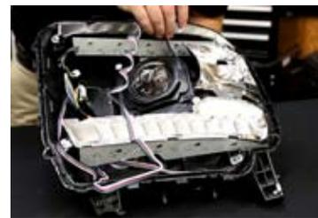
7. Run the RGBW ribbon cable out of headlamp, sealing any hole that you may create. Replace the headlamp lens and repeat for the other side.
