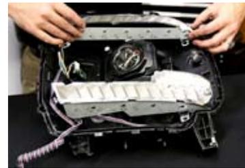
6. After ensuring the epoxy is completely dry, reinstall the reflector housing units. Then reinstall the turn signal housing and replace all the original screws.
