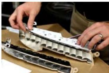
3. Remove any shavings from the reflector housings. Using the original plastic rivet points, place the new Diode Dynamics LED boards into position.
