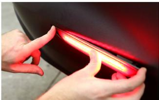
4. Finish your installation by sliding and clipping your new LED sidemarker into place. Be sure to tuck all wiring away from any heat element, including the exhaust.
