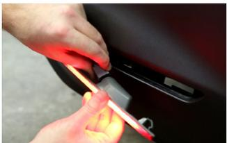
3. Insert the socket into your new sidemarker housing. Be sure to push the connector all the way into the housing.
