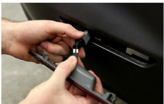
2. Next, remove the factory sidemarker by reaching behind and depressing the tab on the side closest to the wheel well. Once the tab is unclipped, slide the sidemarker towards the wheel well to pull the sidemarker housing out. Set the factory sidemarker aside. It will not be reused. Plug the LED sidemarker into the wiring harness.
