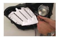
7. Run RGBW ribbon cable out of headlamp, along with the 6-lead sequential connector, sealing any holes that you may create.
