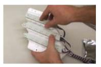
4. Place the new Diode Dynamics LED boards into position. All holes should align perfectly. Due to the larger footprint of the new LEDs, the panels will not push down fully in place. One of the LEDs in each segment may be partially obstructed by the white housing. This is normal fitment, as intended.
