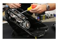
Remove the factory LED panels by unscrewing the screws holding the reflector housing in place and then unclip the wire connector.
