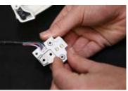
4. Once all the screws are removed, pull the factory board off. Leave the thermal adhesion tape (sil-pad) on the heat sink. This will be reused.
