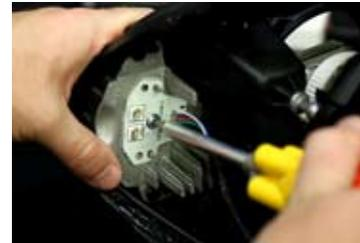
4. Using the alignment tabs, place the new board into place and replace the original retaining screw. Next, replace the black alignment bracket using the original screws. **DO NOT OVERTIGHTEN.**
