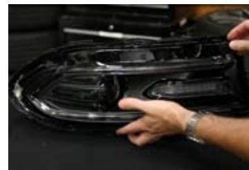
7. Using the alignment tabs, reinstall the black bezel. Once complete, replace the original torx screws and headlamp lens. Repeat for other headlamp.
