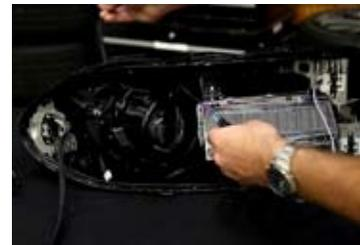
6. Once complete, route the ribbon cables out of the headlamp through the dust cap, sealing any holes that you may create.
