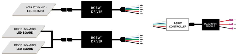
**IMPORTANT: DO NOT plug the LED panel directly into controller without the driver. The LEDs must be plugged into driver first to control the power.**
