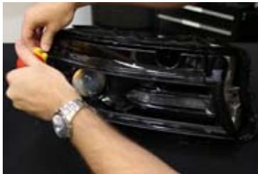
1. First, access the factory LED panels by removing the 4 screws holding the black bezel in place using a T20 bit. Once removed, pull the bezel off and set it to the side.
