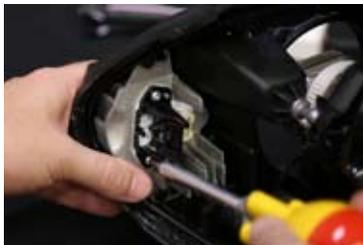
2. Next, remove the torx screws holding the black alignment bracket in place over the factory boards. Pull the bracket off and unclip the power connector from the factory board. Remove the final torx screw holding the factory board in place.
