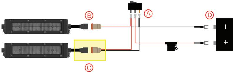
1. Determine a suitable location to mount the switch and route the switch to that location. This may require going through the vehicle's firewall. We recommend unplugging the toggle switch from the harness to route the wires more easily. Drill an appropriate-sized hole for the switch. Then reconnect the wires to the switch and mount it **A**.
