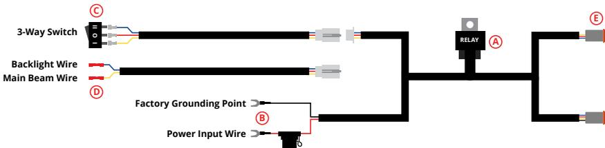
1. Determine a suitable location to mount the relay, (A) near the battery or main power terminal.
