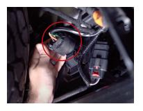
1. Disconnect the plug on the back of the 7-pin trailer connector, by reaching up underneath the bumper. Depress any locking tabs and slide the connector off. Connect the provided wire harness in-line, by connecting one side to the original plug, and the other side to the back of the 7-pin connector.
