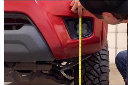
11. On your vehicle, measure the distance between the ground and the center of your SS3 pod. This is your mounting height.
