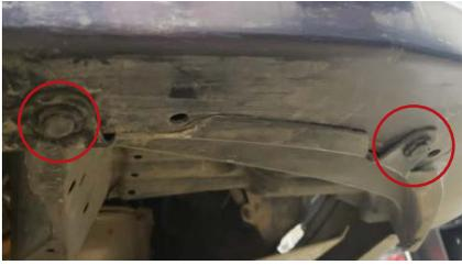
3. Remove the two push clips securing the fender liner to the bottom of the bumper.
