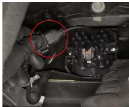
5. Plug the SS3 into the factory fog light harness using the included DT wire adapter. Test function. If the light does not turn on, try flipping the connector 180°.
