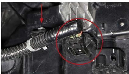
2. Access your factory fog lights. Unplug the fog lamp connector and free the harness from the retaining clip using a flathead screwdriver.
