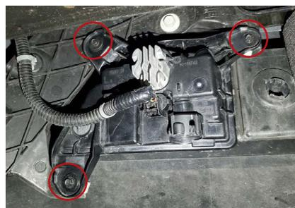
3. Use a 7mm socket and ratchet to remove the three bolts holding the factory fog light housing in place, as shown in the picture to the left. Remove the factory fog light housing. The factory bolts will be reused.
