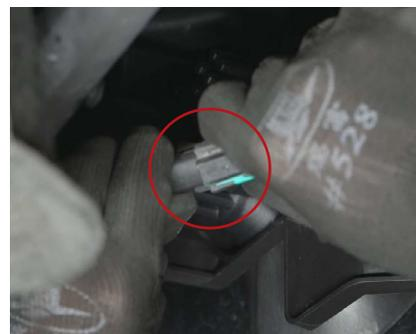
5. Plug the SS3 into the factory fog light harness using the included Molex wire adapter.
