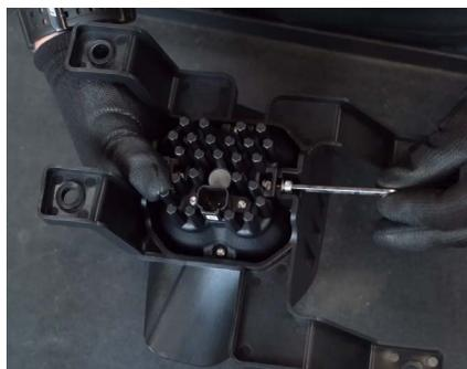
1. Install the supplied nuts into the pod housing with the nylon facing inward. Attach the bracket to the pod using the supplied screws and washers. Make sure the bracket is in the correct orientation. See diagrams above. Ensure that the screws are tightened such that the pod retains its position, but can pivot with force for aiming.
