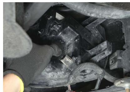
3. Use a 7mm socket and ratchet to remove the four bolts holding the factory fog light housing in place. Remove the factory fog light housing. The factory bolts will be reused.
