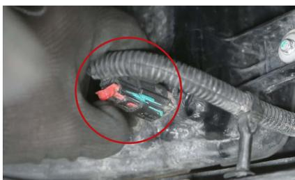
2. Access your factory fog lights and unplug the fog lamp connector, as shown in the picture to the left.
