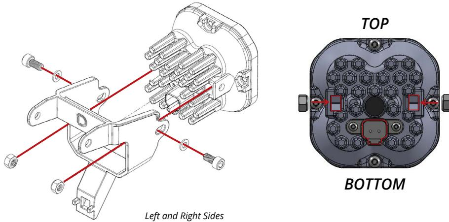
6. Install Type SDX bracket and SS3 assembly onto the vehicle. Plug in the included DT to H10 adapter, and pass it through the opening in the rear of the OEM lamp bracket. Reuse the OEM plastic push-rivets on the top of the bracket. Reinstall the OEM lamp bracket if removed in step 3.
