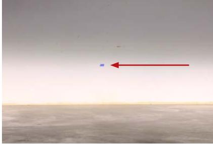
13. Aim your SS3 pods on each side, so that the top of the beam pattern is on the cutoff line mark. To do so, use a 8mm socket to tighten the adjustment screw until satisfied with the beam position.
