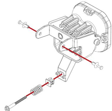
7. Using an 8mm socket, install the OEM aim adjustment screw and compression spring as shown to the left.
