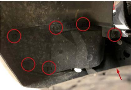
3. Remove the plastic fog light covers. To do so, use a 7mm socket and ratchet to remove the seven screws shown in the picture to the left.
