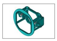
3. Place the included plastic spacers just inside the outer tabs of the SS3 bracket, on each side. Spacers are shown in grey color in diagram above.
