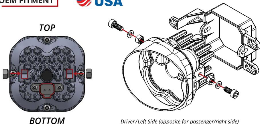
1. Install the supplied nuts into the pod housing with the nylon facing inward. Attach the bracket to the pod using the supplied screws and washers. Make sure the bracket is in the correct orientation, and the lamp angle matches the bracket. The side of the vehicle is indicated on the back of the bracket. See diagrams above. Ensure that the screws are tightened such that the pod retains its position, but can pivot with force for aiming.
