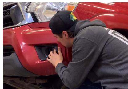
8. Loosen the 5/32" allen bolts on each side of your SS3 pod, just enough to allow you to adjust the pod.
