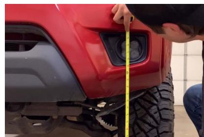
9. On your vehicle, measure the distance between the ground and the center of your SS3 pod. This is your mounting height.
