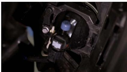
2. Access your factory fog lights. Usually it is easiest to pull back the wheel well liner and reach to the lights.
