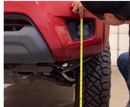
8. On your vehicle, measure the distance between the ground and the center of your SS3 pod. This is your mounting height.
