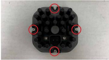
1. Remove the front bezel from the pod by placing the SS3 face down and removing the four T10 Torx screws. Repeat for the second pod.
