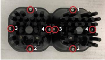
5. Using the T10 screws provided with the frame, tighten them in a "plus pattern" (top-bottom-left-right) to ensure the o-ring around the optic creates an even seal with the frame.
