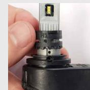
**3. Pull the inner collar up and off the bulb. Take note of how the inner and outer collar interlock with each other. If the two parts are tightly joined, remove both and pull apart.**
