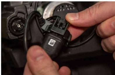
**4. Plug the SL1 connector into the factory electrical socket.**
