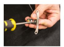
1. If applicable, attach the Demon Eye to the top of the Mini H1 bracket, using one of the included locking screws and locknuts. Ensure the locknut is on the bottom side of the Demon Eye. Be sure to thread the locking screw and locknut first and then tighten using pliers and a small Philips screwdriver.
