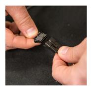
3. Connect the Demon Eye to the Driver. Next, connect the Driver to your RGBW controller. Your controller should be powered to any 12V power source and ground.
