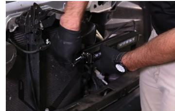
4. Using the included hardware, attach your 12" Stage Series light bars to the brackets, only hand-tightening them.
