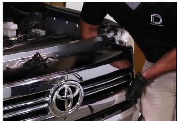
2. Next, reach behind the headlight to a long pointed tab holding the bottom portion of the grille in place. Push down on the tab while pulling forward on the grille to release it. Repeat the same process for the other side of the truck and then set the grille aside on a soft surface.
