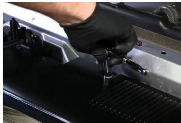
1. Using a 10mm socket wrench and plastic trim removal tool, remove the four 10mm bolts and two plastic rivets located on the edge of the grille inside the engine bay.
