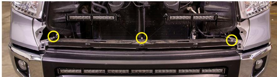
3. Locate and remove the 10mm bolt in the center and two 10mm bolts on the sides. See image above. Using the factory mounting points, mount the brackets using the bolts that you just removed.
