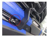
5. Install the SS5 support bracket through the grille opening where the horizontal piece was removed in the previous step. Using a 10mm socket, hand tighten the SS5 support bracket to the base bracket using the two M8 bolts, washers, and nuts.
