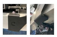
3. Install the base SS5 bracket over the bumper support and secure it using the original bolts removed in the previous step. Ensure the DD logo is in the correct orientation. Do not overtighten the bolts.
