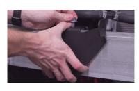
8. Install your new light bar bracket over the crash bar and secure it using the original bolts removed in the previous steps. Ensure the DD logo is in the correct orientation. Do not tighten the bolts.
