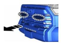
5. Pull out on both sides to release clips holding the grille in place. Then remove the front grille/bumper assembly by pulling forward.
