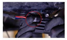
14. Plug the DT connector into the back of the pods and the amp connector into the provided universal harness coming from the taillight **D**.
