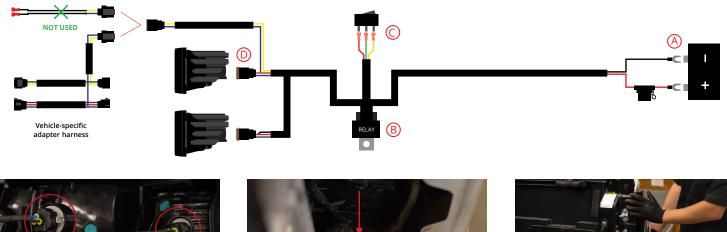
7. Connect the provided vehicle specific adapter harness in-line in between the connector on the OEM harness and the connector on the back of the taillight.
