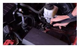
13. Route the connector end of the harness down underneath the vehicle however you see best fit. For this application, we recommend following the wheel well underneath, making sure to avoid any hot or moving parts.
