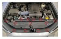
10. Reinstall the core support trim panel using the original thirteen push-rivets. Push the center of the push-rivets down so that they are flush with the top of the surface to lock them in place.
