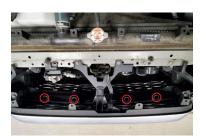
2. Using a trim removal tool or flathead screwdriver, remove the four plastic push-rivets shown in the image to the left.
