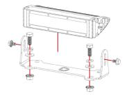
4. Using a 10mm wrench, install your Stage Series 6" light bars in the brackets with the provided M6 hardware.
