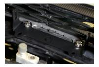
3. Install your new Diode Dynamics brackets using the provided M8 hardware in the newly uncovered holes shown in the image to the left.
