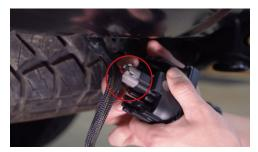
14. Plug the DT connector into the back of the pods and the amp connector into the provided universal harness coming from the taillight ①.
