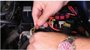
7. Connect the module from the wiring harness to the spade connectors on the fuses Ⓐ. Connect the red wire to the 15A high beam fuse (fuse 7) and the white wire to the 30A low beam fuse (fuse 6).
