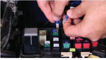
6. Reinstall the fuses back into the fuse box, ensuring the 15A fuse goes into the high beam slot (fuse 7) and the 30A fuse goes into the low beam slot (fuse 6).
