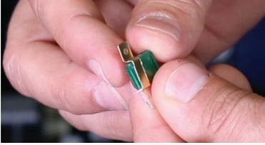
5. Install the included spade connectors onto both fuses. To do so, line up the slot with one of the spades on the fuse and slide the spade connector over to lock it into place. Repeat the process for the other fuse.
