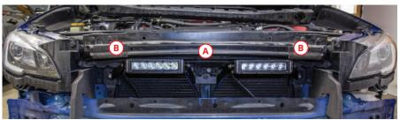
4. With the bumper removed, locate and remove the 12mm bolt (4) in the center and the two 10 mm bolts on the sides 8.
