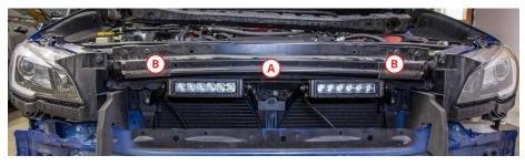
4. With the bumper removed, locate and remove the 12mm bolt (a) in the center and the two 10 mm holts on the sides (B).
