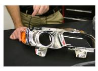
4. Install your new Diode Dynamics C-Light by running the wires through the hole where the factory bulb was and setting the LED board into place.
