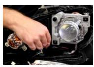
6. Reinstall the chrome housing back in the headlamp assembly by running the wires through the dust cap, sealing any holes that you may create.
