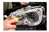
7. Using the alignment tabs, replace the five original screws. Once complete, replace the headlamp lens and repeat for other headlamp.
