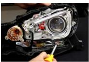
1. To begin, remove the lens. Then remove the five screws holding the chrome housing in place.
