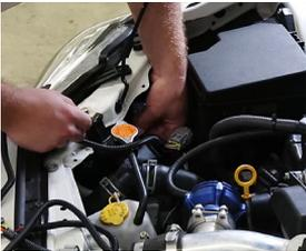
**3.** Unplug the headlight connector on one side of the vehicle and plug the new headlight module inline, between the headlight and vehicle harness connectors. Repeat the process for the other side of the vehicle.
