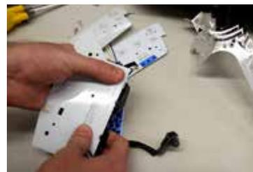
5. Install your new Diode Dynamics LED boards by snapping the large board into the black plastic holder.
