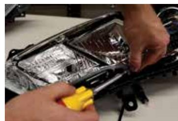
7. Route the switchback wire through the grommet in the headlamp by pushing the grommet to the side and feeding the wire through. Using the alignment pins, reinstall the reflector housing back in the headlamp ensuring any extra wires are out of the way and the light pipe is back in its original position. Replace the original screws. Finally, replace the lens and repeat for the other side.
