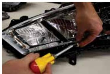
1. Remove the lens. To access the factory LED panels, remove the 3 Phillips screws holding the panels to the black plastic housing.
