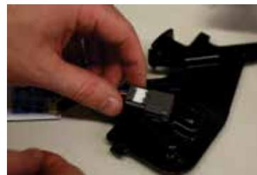
4. Next, remove the large panel from the black plastic holder it is attached to. The black plastic holder will be reused. After that, remove the large panel connector from the black plastic holder by depressing the large tabs on the gray connector.
