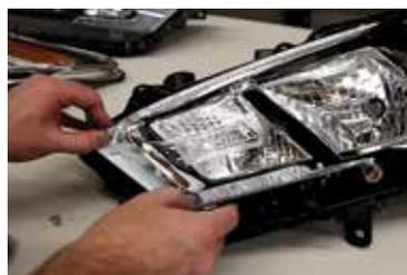
2. Unclip the factory connector and pull the LED panel housing straight out to remove it. Set the rest of the headlamp housing aside.
