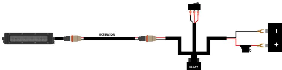
5. Determine a suitable location to mount the switch and route the switch to that location. We recommend unplugging the toggle switch from the harness to route the wire more easily. If needed, drill an appropriate-sized hole for the switch. Then reconnect the wires to the switch and mount it.
