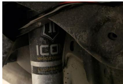
11. Route the wire in front of the rear shock and through the opening toward the back of the vehicle. Next, route the wire from the rear fender liner into the rear bumper, pulling any remaining slack.
