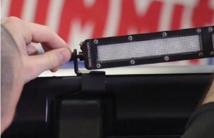
3. Close the hatch and mount your light bar to the brackets using the included 10mm bolts.
