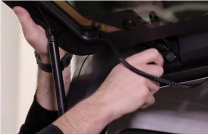
2. Using one hand to support the back glass, set the bracket into place. Then reinstall the 10mm bolts. Repeat for the other side of the vehicle.
