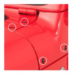
1. On the driver side, remove the four bolts on the cowl as shown in the picture to the left using a T40 Torx bit and ratchet.
