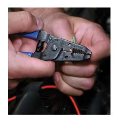
7. Locate and connect to one of the four power wires for the Auxiliary Switch Bank near the battery. Using wire strippers, remove enough insulation to make a good connection. Insert the yellow wire into the butt connector and crimp it to secure the connection.
