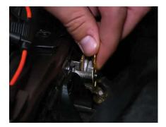
9. Connect positive and negative battery wires to the battery, or to main power terminals near the fuse box.
