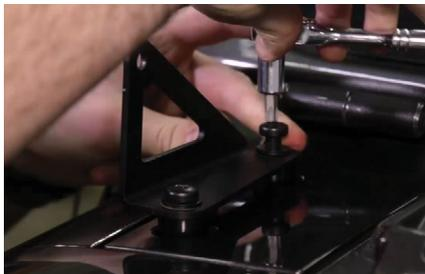
3. Align the bracket in place, and use the included OEM-style extended hardware to secure. Repeat for the other side of the vehicle.
