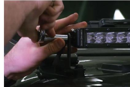
4. Mount your 50" light bar to the brackets using the low profile hex bolts included in the universal mounting bracket box. Secure using a 10mm socket.
