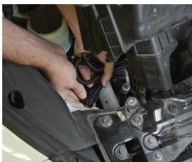
5. Then plug the larger set of connectors on the new module inline, between the headlight and vehicle harness connectors. Run the remaining connectors down to the fog light location.
