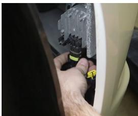
6. On the passenger side of the vehicle, remove the locking screw in the wheel well. Pull the fender liner back slightly to access the fog light connector. Pull back on the tab on the fog light connector to release it. Then plug the rest of the module in line. \*\*\*If the vehicle has the optional adaptive lighting feature, you may need to reach around or underneath the adaptive lighting controller to access the fog lamp.
