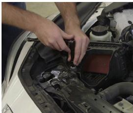
3. On the passenger side of the vehicle, remove the two 10mm screws holding the air box in place. You may need to gently lift up on the shroud cover to access the second screw. After both screws have been removed, pull the air box straight up and set it to where you can gain access to the headlight connector.
