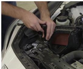
3. On the passenger side of the vehicle, remove the two 10mm screws holding the air box in place. You may need to gently lift up on the shroud cover to access the second screw. After both screws have been removed, pull the air box straight up and set it to where you can gain access to the headlight connector.
