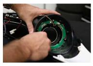
2. Next, remove the three screws holding the factory board in place.
