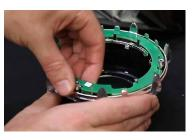
5. Pull straight up on the factory board to remove it
