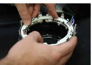
6. Using the alignment notches, place your Diode Dynamics board in place. Next, replace the shroud in the main bezel and clip into place. Ensure the wiring is on the upper left hand side when looking at the front of the assembly. Replace the original screws.
