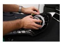
7. Reinstall the main bezel back in the headlamp housing. Run the RGBW ribbon cable out of the headlamp, sealing any holes that you may create. Replace the headlamp lens and repeat for the other side.
