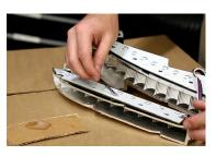
4. Fix the new panels in place by applying 5-minute epoxy to completely cover the plastic rivets tabs. The epoxy should create a bond between the plastic rivet point and the board. Use enough epoxy so that there is a bond all the way around each rivet, contacting the board fully.
