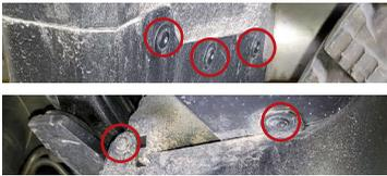
**1.** Using a T15 Torx driver, remove the five screws from the mud flap in the rear wheel well.
