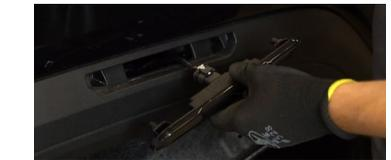
**12.** Plug in your new sidemarker and move the locking tab to the locked position.
