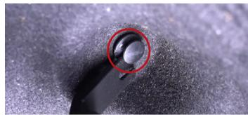
**3.** Using a trim removal tool, remove the one plastic push-rievet from the fender liner. Remove the fender liner from the vehicle.
