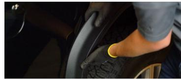
**3.** Using a trim removal tool carefully pry the rear fender flare off the bed. It is held in place by 22 plastic clips.
