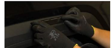
**11.** Using a T20 Torx driver and original hardware, install your new sidemarker in the front fender flare.
