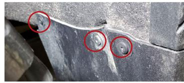
**1.** Using a T15 Torx driver, remove the five screws holding the mud flap in place. There is no need to fully remove it. You may need to turn the wheel to gain access to the screws.
