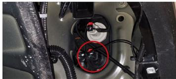
**8.** From the wheel well, unplug the lower black connector from the headlight. To do so, slide the red tab back and then depress the black tab.
