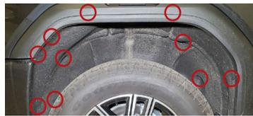
**2.** Remove the ten T15 Torx screws holding the fender liner in place.
