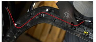
**11.** Pass the adapter harness through the hole in the bed and route along the fender flare using the path of the OEM harness.
