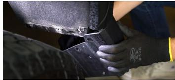
**2.** Remove the rear-most mud flap by pulling down and tilting slightly outboard.
