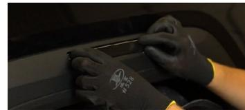
**10.** Using a T20 Torx driver and OEM hardware, install your new sidemarker.
