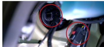
**9.** Plug the headlight connector into the included adapter harness and then plug the adapter harness into the headlight. Be sure to slide the red tab back.
