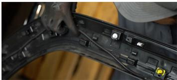
**9.** Remove the OEM sidemarker harness from the fender flare. Pass the OEM harness back through the hole in the truck bed and secure in a bundle with zip ties.
