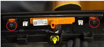
**4.** Using a T20 Torx driver, remove the two screws holding the rear sidemarker in place.
