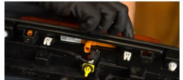
**6.** Remove the sidemarker by pulling it out through the front of the fender flare.
