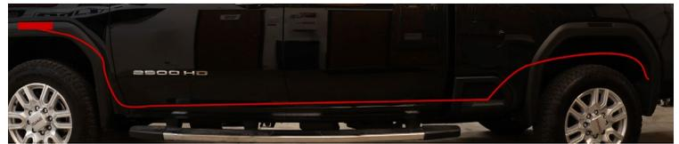
**14.** Route the harness along the frame rail to behind the rear wheel of the truck, securing with zip ties along the way. Ensure the harness passes over the rear axle along the frame rail and is secured such that it cannot get pinched or caught in any moving parts.
