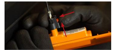
**5.** Remove the sidemarker by pulling it out through the front of the fender flare. Pull the red locking tab back and then depress the black tab to remove the connector.
