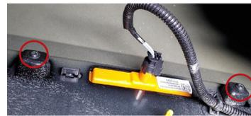
**4.** Using a T20 Torx driver, remove the two screws holding the factory sidemarker in place.
