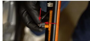
**5.** Pull the red locking tab back and then depress the black tab to remove the connector.
