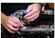
2. After the headlight has been opened, remove the four Phillips screws holding the silver bezel in place. Remove the silver bezel and set it aside on a soft surface.
