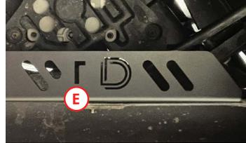
3. Slide the bracket in-between the bumper and the support **E**. Using the stock mounting points, replace the original 13mm screw, only hand-tightening it.
