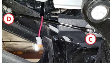
2. Using an 8mm socket, loosen screw **C** from the strut. Do not fully remove the screw. After that, remove screw **D** from the strut.
