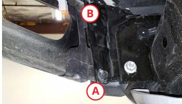
1. Using a 13mm socket, loosen screw **A**. Do not fully remove the screw. Next, remove screw **B**.
