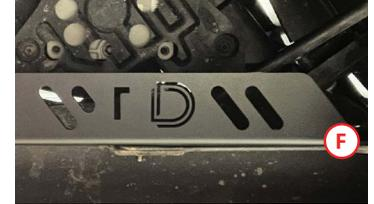
4. Slide the other side of the bracket between the strut and the bumper **F**. Using the stock mounting points, install the included M6 screw, only hand-tightening it.
